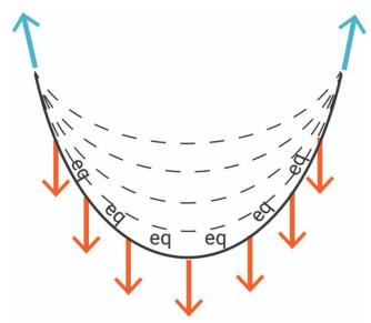
One of the most innovative aspects of the Arch is its unique shape—a catenary curve. This shape mirrors the arc formed when a chain is suspended from both ends, and when inverted, becomes one of the most structurally sound curves in engineering.
