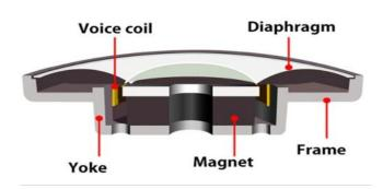
A diaphragm is an important part within every driver unit. It contains a thin membrane which creates audio waves [2]. When the coil vibrates the diaphragm moves with it, this movement causes pressure waves (sound waves). These waves are the sounds you hear. The diaphragm moves quickly for higher pitched sounds and lower/slower for slower pitched sounds [1]. The intensity and direction of movement is directed by the electrical signal which enters the driver. [2]
