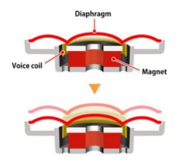
The electromagnetic fields switch their polarity back and forth depending on the pattern it's sent, or the sounds being produced. When the electromagnet switches its polarity, it is rapidly repelled and attracted to the permanent magnet which makes it vibrate. This causes the diaphragm to vibrate [4]. Altering the strength and direction of the electric current causes the diaphragm to vibrate and to produce the sound.
